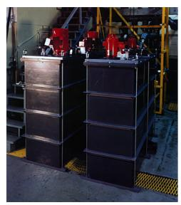
These Vanton PVC tank/pump systems stand 66" high, 78" long and 26" wide. The 48" cantilevered shafts of the two Vanton SGH sump pumps are housed in heavily ribbed PVC columns to provide the extra rigidity required. The pumps are driven by 5 HP, 1750 RPM hollow shaft motors and deliver 120 PGM at 40' TDH.
